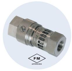
When FireChek senses excessive heat from a nearby fire, it immediately vents the pneumatic actuator and closes the actuator air supply line. FireChek triggers quickly, securing pneumatically operated process line valves. Because FireChek responds to heat, not flame, it offers dramatically improved protection compared with conventional plastic tubing burn-through. It shuts off the air supply line to prevent plant air from feeding oxygen to a fire.
