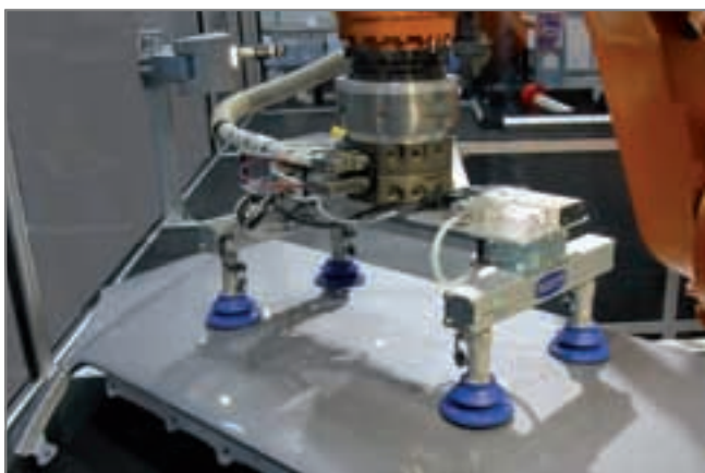
Suction pads with inline valves IV being used for handling car bodywork parts
