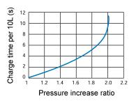
\* When filling tank with air, where Primary side air pressure  $P_0$ , air pressure in tank before filling  $P_1$ , air pressure after filling  $P_2$ , boosting ratio before filling  $K_1=P_1/P_0$  and after filling  $K_2=P_2/P_0$ . Find  $K_1$  and  $K_2$  at first, then read filling time  $t_1$  and  $t_2$  according to graph where boosting ratio  $K_1$ ,  $K_2$ , Finally filling time for tank capacity Q is obtained with
