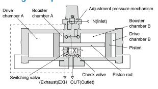
The process described above is repeated to continuously supply highly pressurized air from the IN to the OUT side. The governor establishes the outlet pressure by handle operation and pressure adjustment in the drive chamber by feeding back the outlet pressure.
