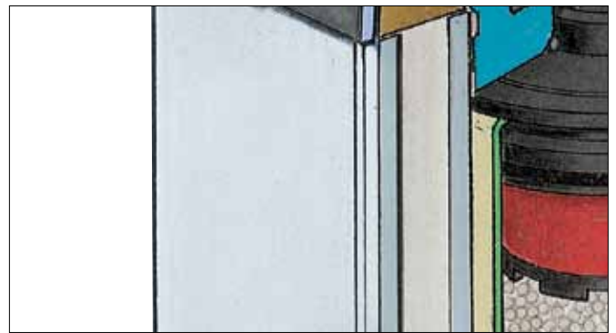
Corrosion protected by alocrom and epoxy painting.
