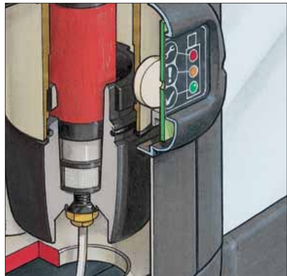
Integral 0.01µm high efficiency filter.
