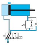
Phase 2: in return direction, pressure is supplied through the control valve
