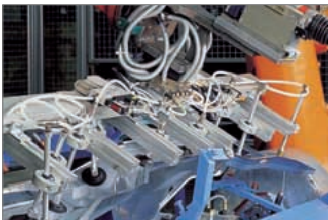
Centralized vacuum generation by means of compact ejectors SCP for handling car body parts
