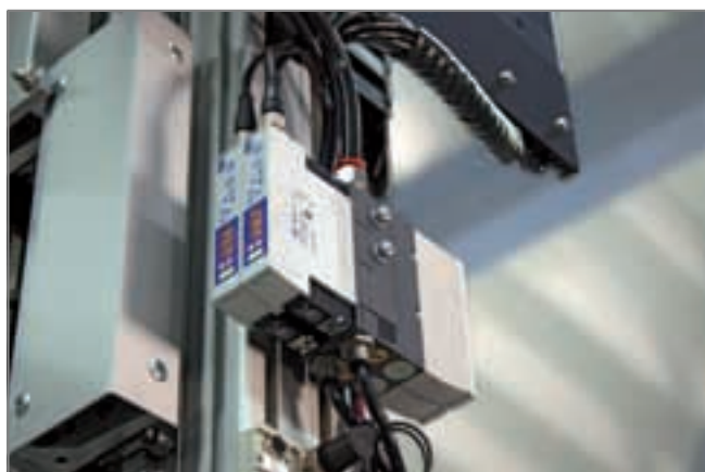
Centralized vacuum generation by means of compact ejectors SMPi
