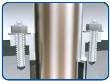
The standard gland packing could provide a good service under high temperature and chemical resistance; on request, the addition live-loading gland can be available for high cycles and low emission service. Special compound of graphite packing materials are also available to provide the low VOC emission, which was verified according ISO 15848-1.
